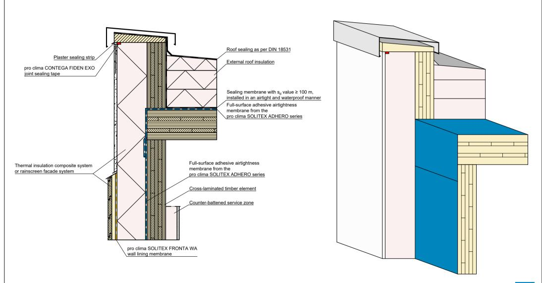
Solid timber construction | Flat roof | SOLITEX ADHERO | Var. 2
