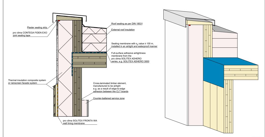
Solid timber construction | Flat roof | SOLITEX ADHERO | Var. 1
